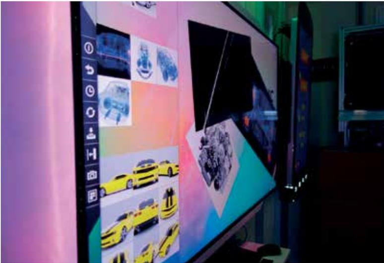
The Zytronic ZXY500 controllers also allow the design of "soft keys" around the edge of the dynamic active area of the projected capacitive touchscreen.
