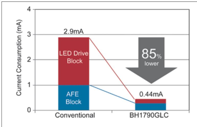
Heart rate sensor current consumption breakdown
