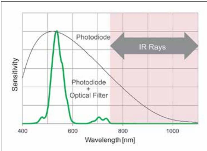
Spectral characteristics of the light receiving block of the BH1790GLC
