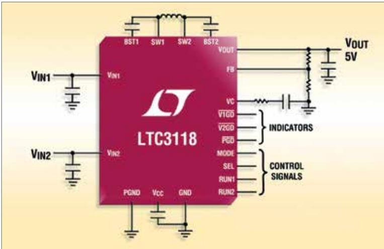
LTC3118 schematic with Power-path section between two inputs
