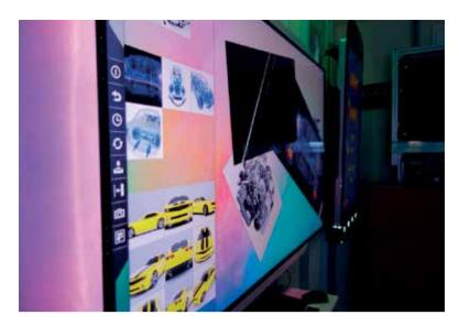
The Zytronic ZXY500 controllers also allow the design of "soft keys" around the edge of the dynamic active area of the projected capacitive touchscreen.
