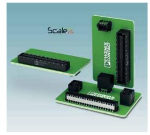
Maximum freedom: Horizontal and vertical female connectors allow mezzanine, orthogonal and coplanar PCB arrangements.
